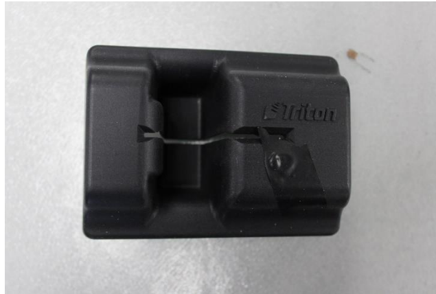
Figure 10. Front view of a skimmer using separate boards for capturing track data and PINs
