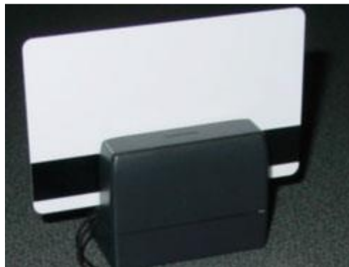
Figure 1. Example of a hand-held skimmer
