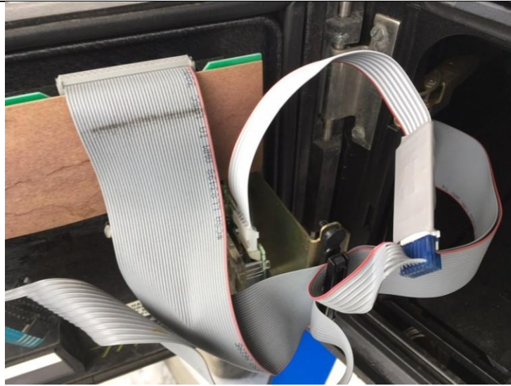
Figure 8. A Bluetooth ® custom skimmer secreted inside a gas pump
